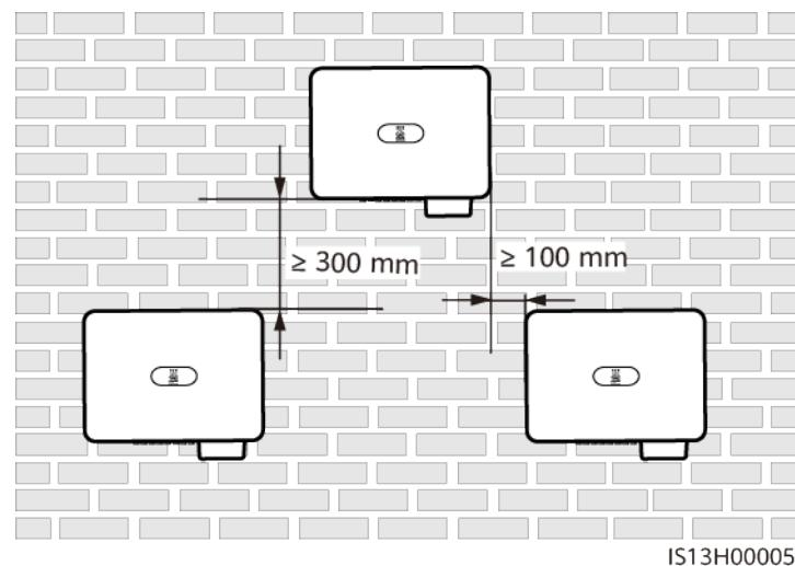
**Figura 4-5** Instalación triangular en tres capas (no recomendada)
