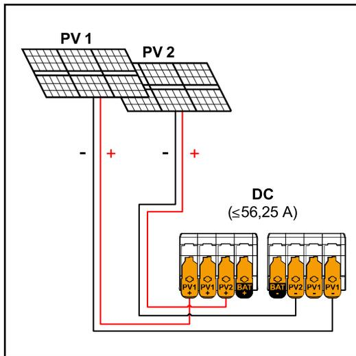
$PV1 (I_{dmax}) = 37,5 A / PV2 (I_{dmax}) = 18,75 A$
